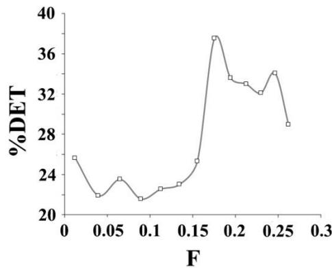
Fig. 5. RQA %DET measures of AE time series of stick-slip process under different external forcings.
