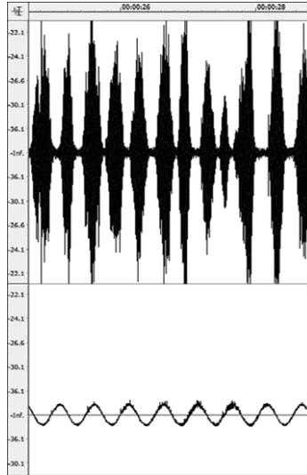
Fig. 1. Typical graph of AE of forced stick-slip. Upper channel - acoustic bursts generated by slips; lower channel – forcing signal.
