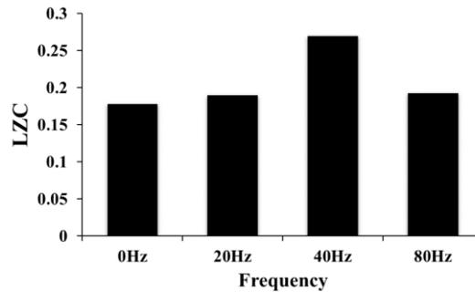
Fig. 3. Lempel-Ziv complexity (LZC) of AE signal recordings of natural (without forcing), 20Hz, 40Hz and 80Hz with applied voltage 1V.
