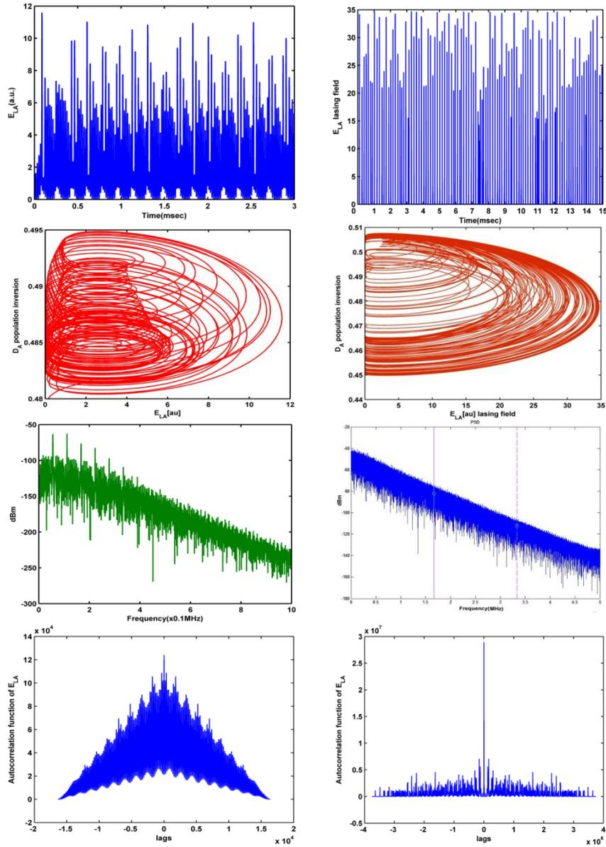
Fig.4 Comparison of quasi-chaos(left) with pure chaos(right) for loss modulation EDFRL
