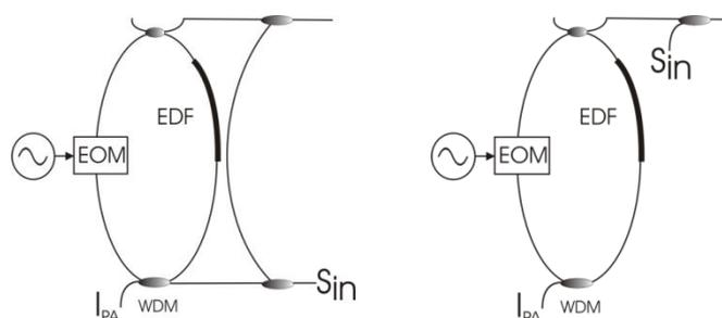
Fig.1 Cavity loss modulation in EDFRL
