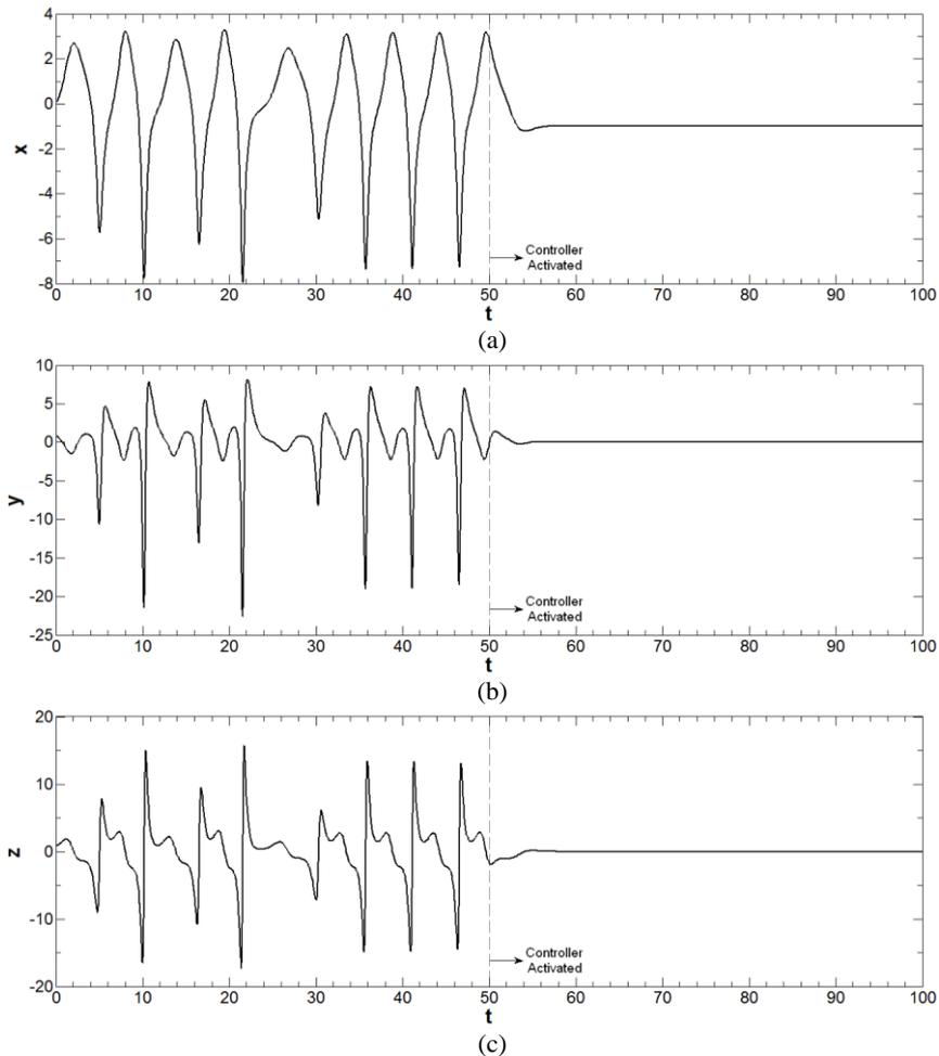
Fig. 6. Time responses of controlled chaotic system having a line equilibrium to  $(-1, 0, 0)$  equilibrium point when the passive controller is activated at  $t = 50$  for (a)  $x$  signals, (b)  $y$  signals, and (c)  $z$  signals.
