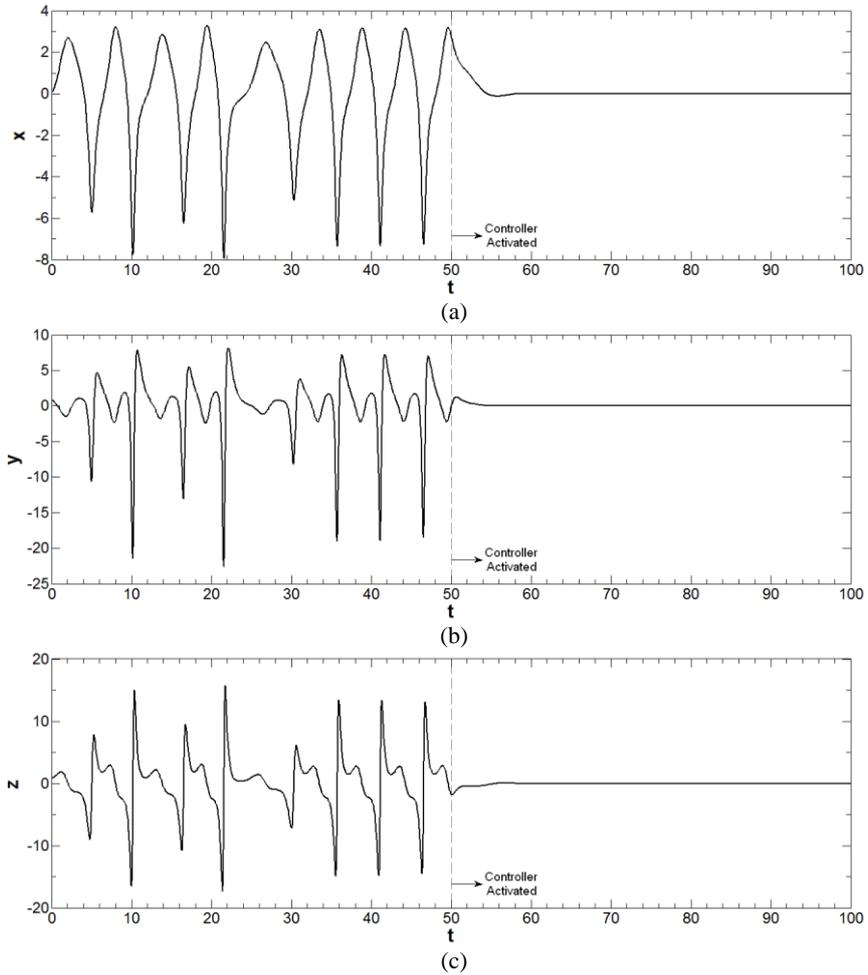
Fig. 5. Time responses of controlled chaotic system having a line equilibrium to  $(0, 0, 0)$  equilibrium point when the passive controller is activated at  $t = 50$  for (a)  $x$  signals, (b)  $y$  signals, and (c)  $z$  signals.
