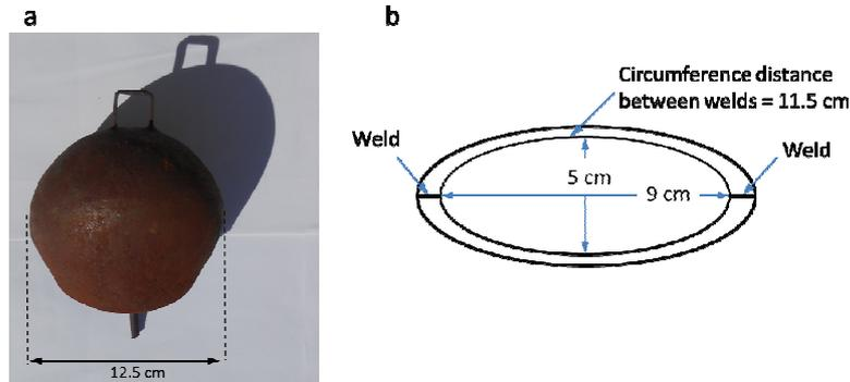
Figure 1a and b: a) photograph of flat side of sheep bell, b) Schematic view of open aperture of sheep bell.
