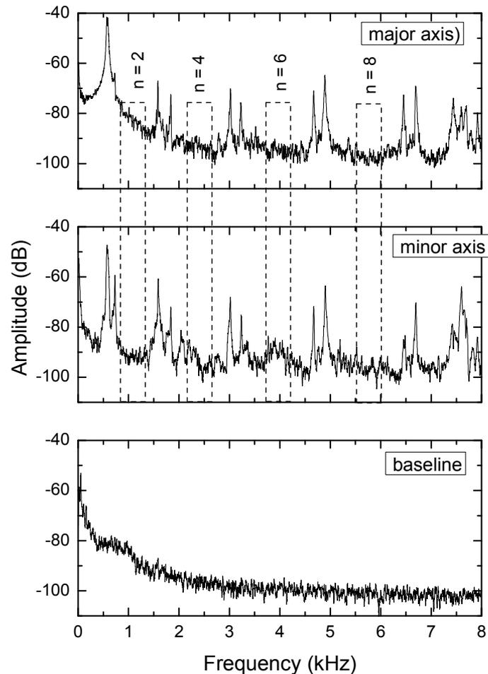
Figure 2: Frequency response of sheep bell as struck on the major, minor axis using a human hand and baseline measurement.
