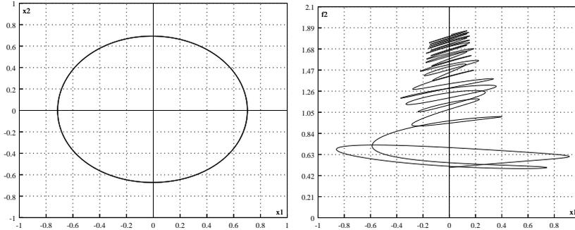
**Fig. 4.** Orbits for the excentric flywheel. Left: capture into resonance ( $x_1 = x, x_2 = \dot{x}$ );  $\phi_1(0) - \phi_2(0) = 1.13, \phi_2(0) = 0, \varepsilon = 0.1$ . Right: transition through the resonance zone, vertical  $f_2 = \phi_2$ ;  $\phi_1(0) - \phi_2(0) = 0.5, \phi_2(0) = 0.5, \varepsilon = 0.1$ .
