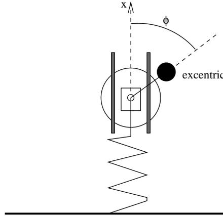
**Fig. 3.** Excentric flywheel, rotating on elastic foundation
