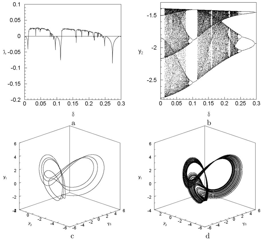
**Fig. 4.** The dependence of maximal non-zero Lyapunov’s characteristic exponent (a), phase-parametric characteristic of the system (b), phase portrait of the limit cycle (c) and the chaotic attractor (d)
