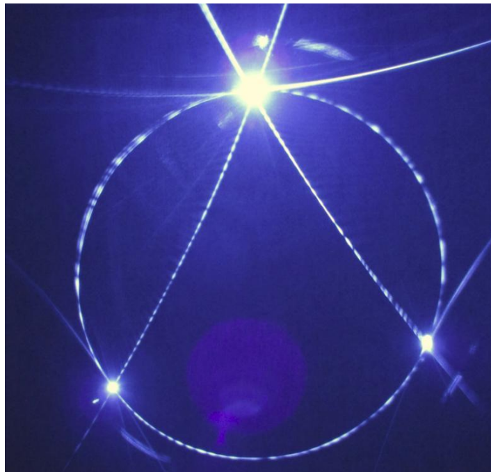
Fig. 6. The parlaseric circle, two laser dogs and laser pillars obtained with blue light.
