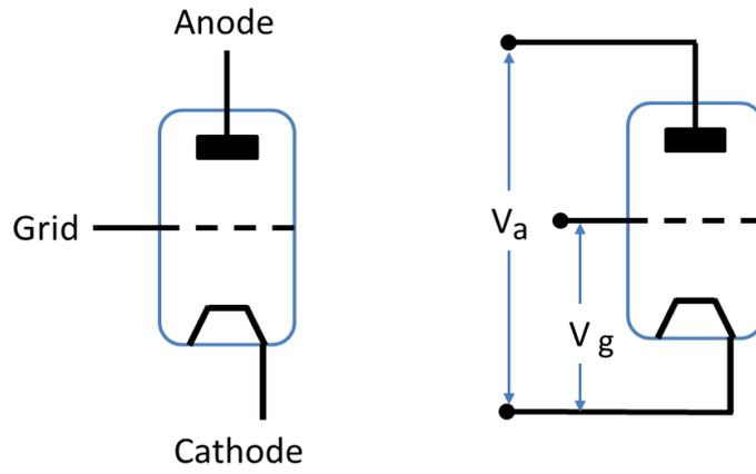
Figure 3. Triode; a) schematic of the triode valve and, b) triode voltage separation between the electrodes.
