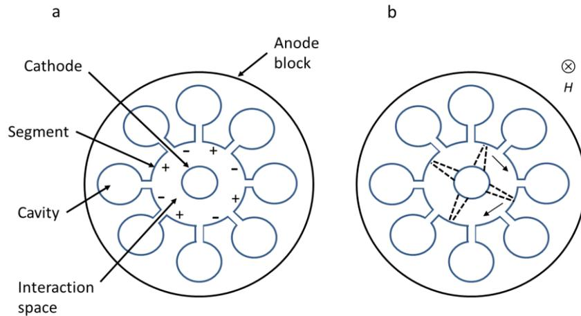
Figure 8. Magnetron; a) cross-section of  $N = 8$  cavity magnetron and, b) the space-charge wheel rotating about the cathode with the magnetic field is going into the page.
