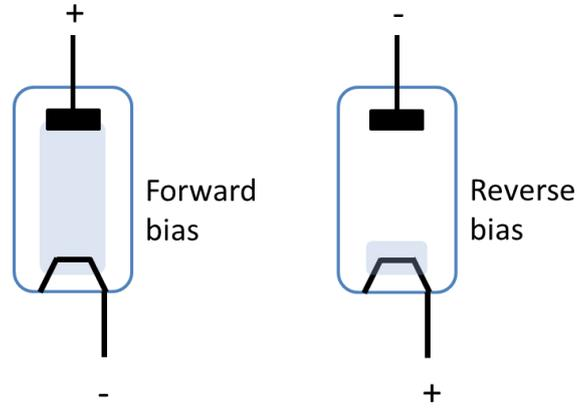
Figure 2. Diode thermionic valve: a) forward bias and, b) reverse bias. Note that the heater is working, and the cathode is heated to incandescence in a high vacuum. The space-charge cloud is shown in blue.
