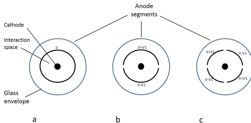
Figure 6. Cross-section schematic of the anode segmentation development. Hull's single anode (a), 2 segment anode (b) and, 4 segment anode (c). The external coil is not shown for clarity.
