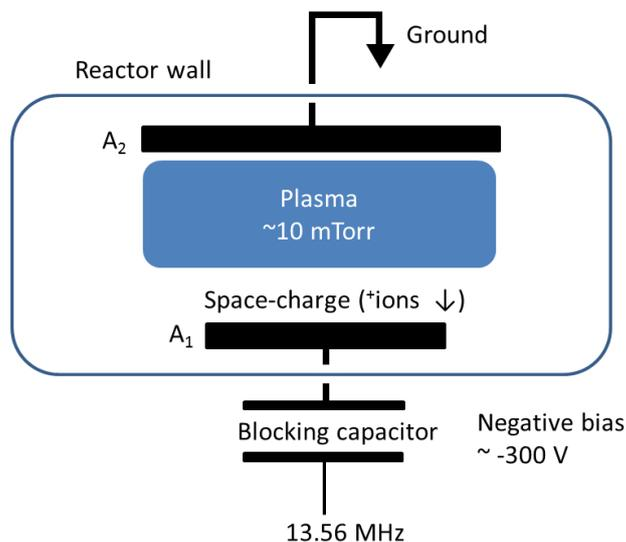
Figure 12. Cross-section of a typical RIE reactor, with external blocking capacitor and driven at 13.56 MHz.
