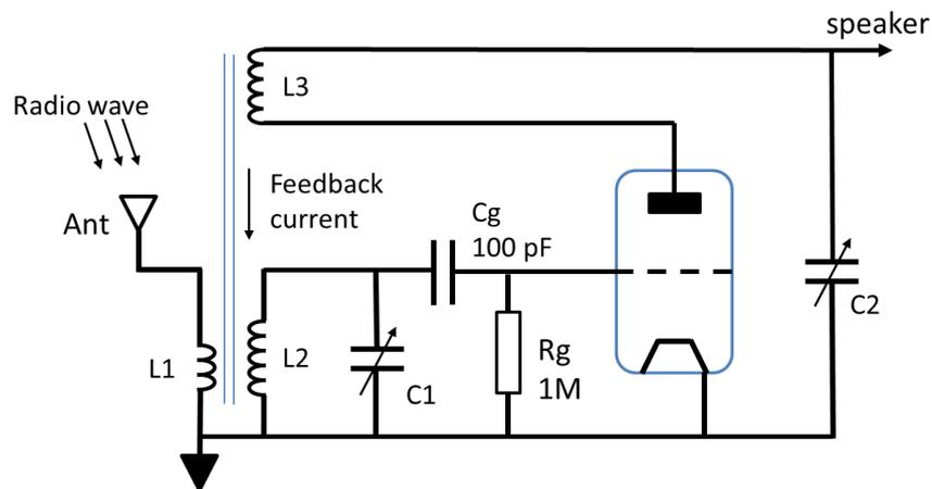
Figure 4. The basic Armstrong regenerative receiver circuit.
