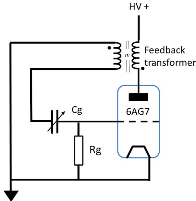
Figure 5. Appleton's triode Squegger oscillator circuit.
