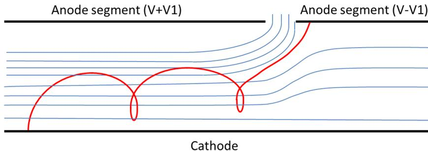
Figure 7. A reconstruction of Heller's simplified scheme of two flat anode segments and cathode. The equipotential lines (fine blue) and electron orbit (thick red) in interaction space are shown.
