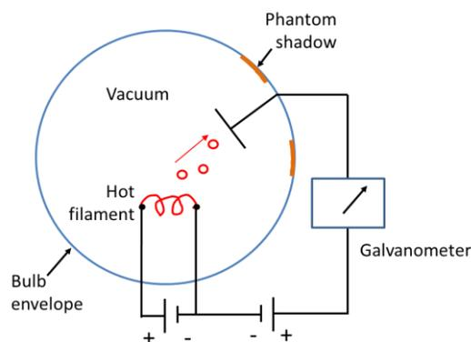
Figure 1. Schematic of "Hammer's phantom shadow" observation and the "Edison effect" measurement.
