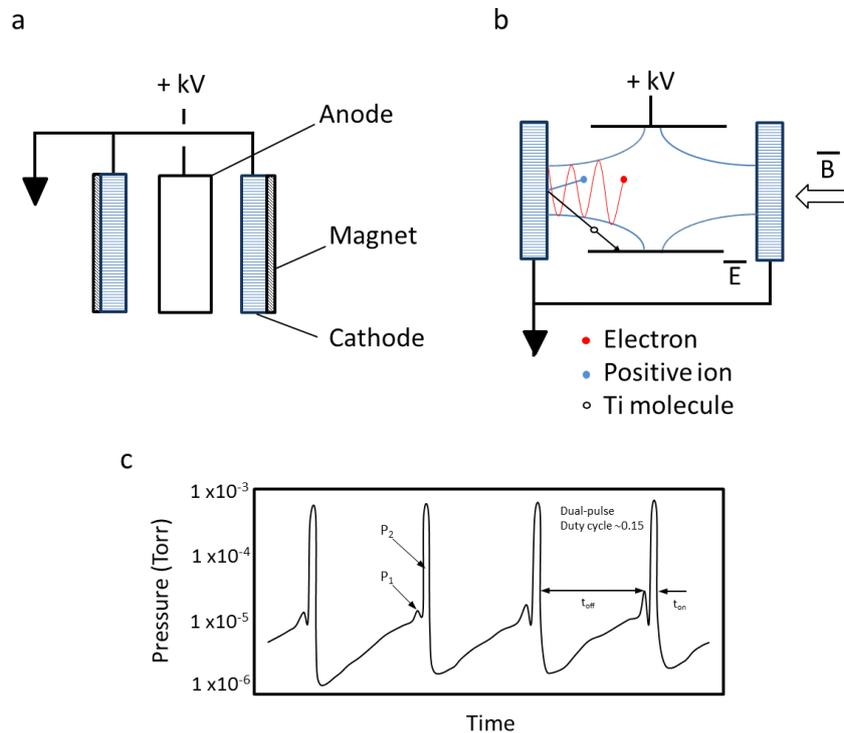
Figure 9. a) cross-section of diode-SIP, b) Penning trap and, c) typical time trace of a cyclic argon instability.
