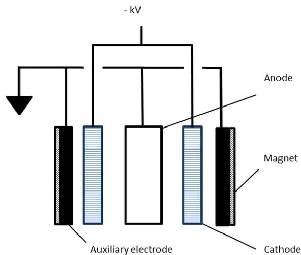
Figure 11. Cross-section of triode SIP.
