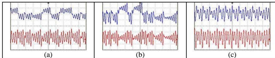
Fig.9. Time domain responses of third nonlinear circuit block in different frequency, x: 2 V/div, y: 0.2 V/div a) time: 2.5 ms/div, b) time: 250  $\mu$ s/div, c) time: 25  $\mu$ s/div.
