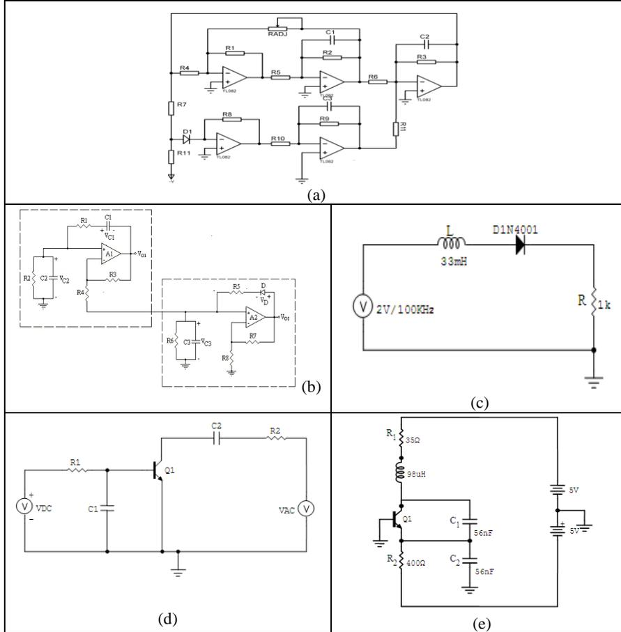
Fig. 3. Chaotic circuits in Chaos Training Board-II; a) Chaotic Rössler Circuit, b) Chaotic Wien Bridge Oscillator, c) Chaotic RLD Circuit, d) Transistor-based Nonautonomous Chaotic oscillator, e) Chaotic Colpitts Oscillator.
