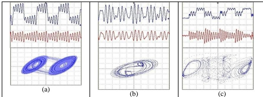
Fig 6. Experimental measurements of MMCC circuit on the board-I; a) with the autonomous mode configuration, b) with the nonautonomous mode configuration, c) with the mixed-mode configuration.
