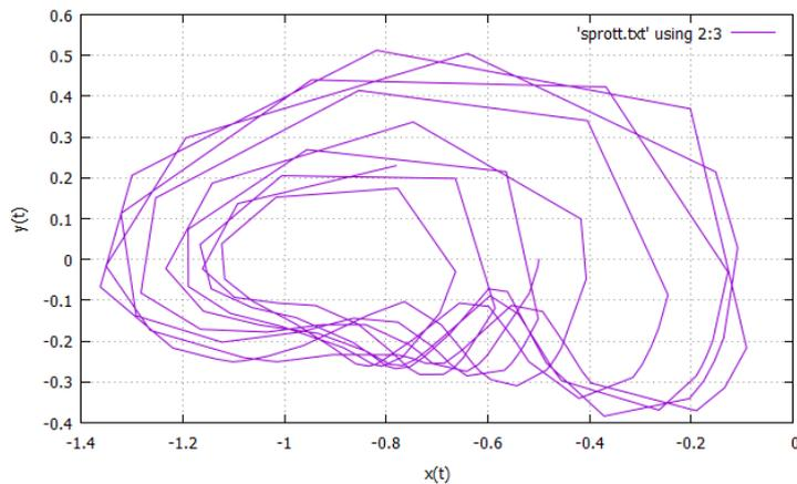
Fig3. Simulation results for Sprott System  $x(t)$  vs.  $y(t)$  with the initial conditions  $x(0) = -0.5$ ,  $y(0) = z(0) = 0$
