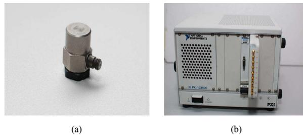
Fig. 1. The data acquisition setup: (a) accelerometer, (b) PXI system.
