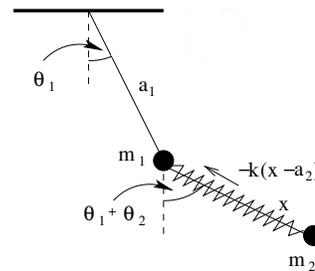
**Fig. 2.** Double spring pendulum.
