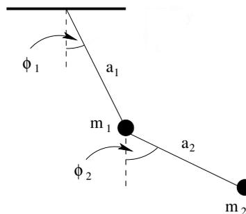
**Fig. 1.** Simple double pendulum.
