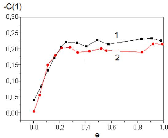
Fig. 7. Magnitude of the correlation factor  $C(1)$  in the resonant cavity as a function of deviation  $e$  from the fully symmetric position of the inner spherical ball (curve 1) or disk (curve 2).
