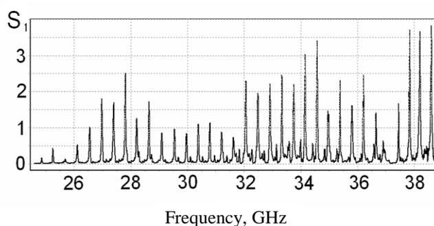
Fig. 2. The spectrum of a spherical resonant cavity with a symmetrically disposed inner sphere.  $S_1$  is the spectral line intensity.
