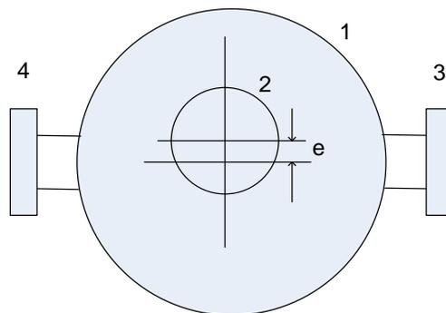
Fig. 1. Schematic of a 3D-resonator with an inner metal sphere: 1- spherical cavity; 2- inner metal sphere; 3 and 4- waveguide / dipole coupling elements for the resonator;  $e$  - eccentricity.
