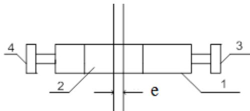
Fig. 6. Schematic of the 2D (cylindrical) volume resonator: 1- casing; 2-inner metal disk; 3 and 4-elements of resonator-to-load diffractive coupling.  $e$  is a measure of eccentricity in the position of the disk in the resonant cavity.
