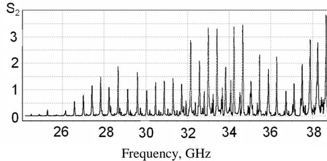
Fig 3. The spectrum of a spherical resonant cavity with a non-symmetrically disposed metal sphere inside.  $S_1$  is the spectral line intensity.
