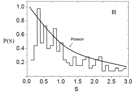
Fig 4. Histogram of interline frequency intervals in the spectrum of a spherical resonator with a symmetrically positioned metal inner sphere;  $s$  is the interline frequency separation, normalized to the mean value, and  $P(s)$  the probability for an interval to fall into a prescribed range.
