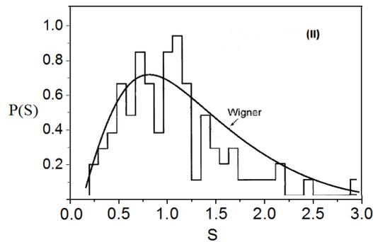
Fig 5. The histogram of interline frequency intervals in the spectrum of a spherical resonator with a non-symmetrically disposed metal inner sphere
