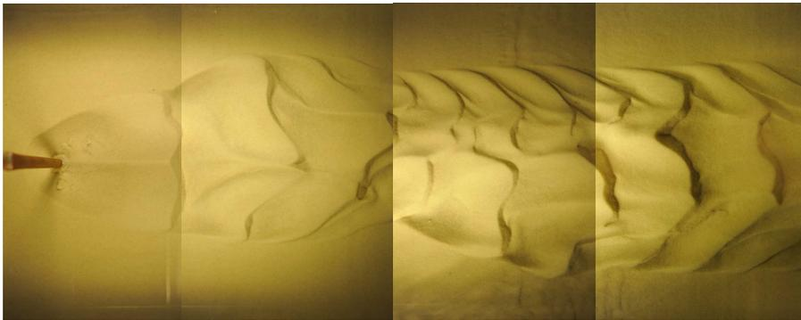
**Fig. 4.** Sedimentary structures downstream the cylinder;  $Re=42000$  (Test 2)
