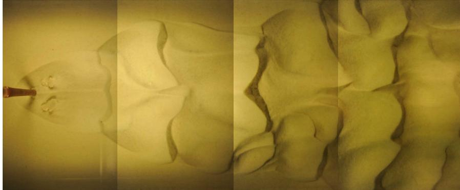
**Fig. 5.** Sedimentary structures downstream the cylinder;  $Re=43000$  (Test 3)
