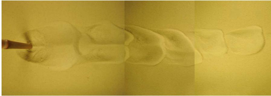
**Fig. 3.** Sedimentary structures downstream the cylinder;  $Re=38000$  (Test 1)
