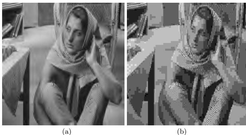
**Fig. 3.**  $256 \times 256 \times 8$  bpp test images used in our experiments ((a) EZW Shapiro (9,7) and (b) JPEG compression are used).
