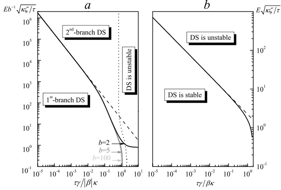
**Fig. 1.** Master diagrams of DS for the normal (*a*) and anomalous (*b*) GDDs. The solid curves correspond to the DS stability thresholds obtained from the variational approximation. The dashed curves correspond to the asymptotic  $c \equiv \tau\gamma/|\beta|\kappa \ll 1$ . The dotted curve in (*a*) corresponds to the stability threshold of the second DS branch with  $\theta > 1$  in (9).
