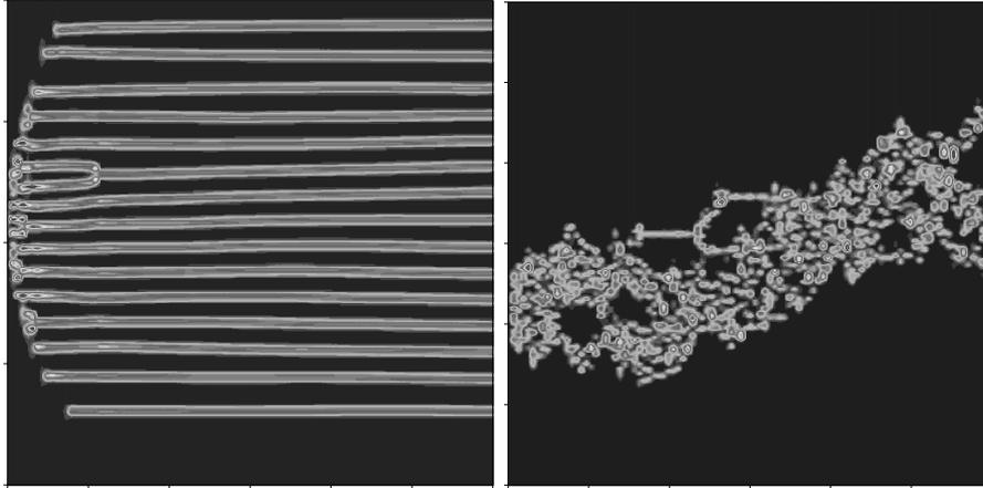
**Fig. 2.** Multiple-pulse complexes (contour plot with brighter regions corresponding to higher powers) in the anomalous GDD regime. Regular multi-pulsing (left) and structural chaotization (right) with approaching the GDD to zero are shown. The axes are  $t$  (vertical) and  $z$  (horizontal).
