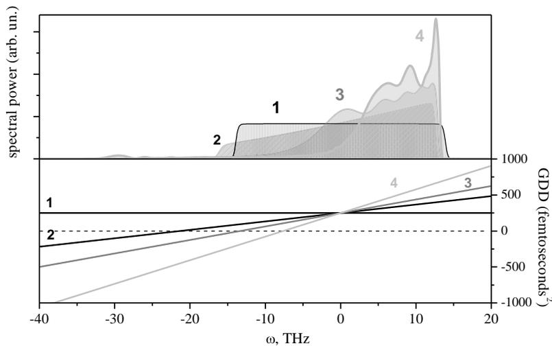
**Fig. 5.** Spectra of the chirped DSs corresponding to the different net-GDD. The GDD slope depends on the TOD value. Here, the positive GDDs correspond to the normal dispersions.
