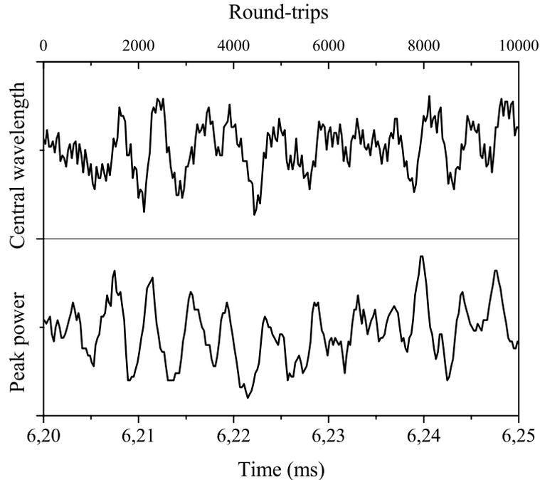
**Fig. 6.** Jitter of the DS central frequency and its peak power due to resonant interaction with the continuum.
